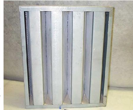
All **DISCARB** products may be supplied with a single face seal on request. As the product is omni-directional in terms of airflow, this suffices as either a clean or dirty air side gasket. If required two gaskets can be fitted. **Discarb** units may be supplied as standard capacity units with 20mm panels or heavy Duty in which case 25mm thick carbon panels will be fitted.
